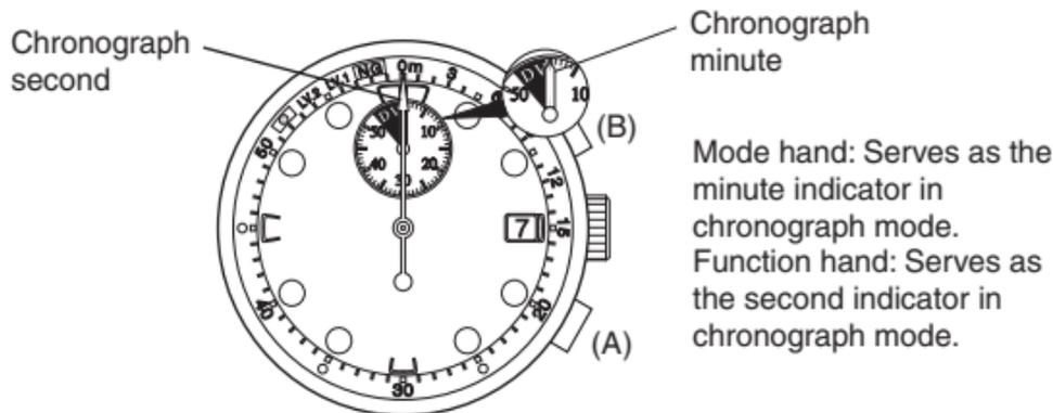
\* If the watch is left in reset status in the chronograph mode for 3 minutes, it automatically switches to the time mode.
