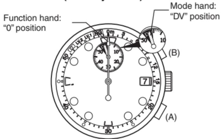
\* If the function hand and mode hand don't point to their respectively specified positions (mode hand: "DV" position, function hand: "0" position) when the watch enters the dive mode (standby status), adjust the hand positions referring to "9. TROUBLESHOOTING".
