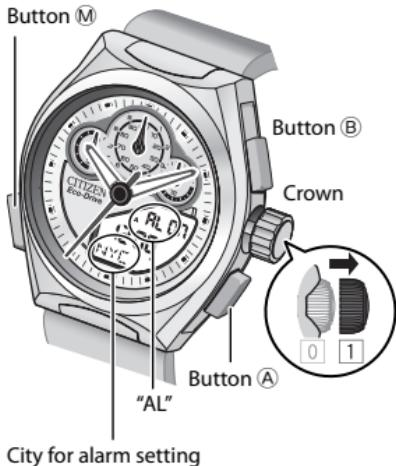
To monitor the alarm sound, press and hold **button A** for more than 2 seconds while **the crown** is set to position ①. You can monitor it for up to 10 seconds.
