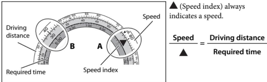
In the circle A, the speed index points to “80.” Then any other part indicates a pair of driving distance and required time with the speed of 80 km/h. When the driving distance is 400 km (“40”), for example, the required time is 5 hours (“5:00”).
